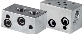
**Pilot operated check valves** can be integrated within modular manifold blocks for NG6 (Cetop 3) valves, thus avoiding the extra modular Cetop 3 sandwich type valve between the base block and the spool valve
