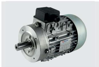
**B14 IEC motors:** for market compatibility, any IEC standard B14 AC motor with frame 63, 71, 80, 90, 100 or 112 can be mounted. These motors are normally procured and mounted by the customer himself. Two-piece couplings and additional adaptor flanges as per following tables must be fitted. Hydrorit can supply frame 112 B14 AC 3-phase motors
