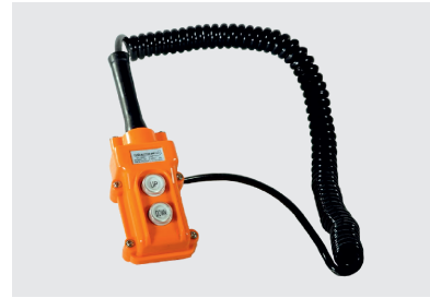
Wired remote control Weight: 0,60 kg Max Current @ Voltage: Protection degree: IP65 2A@400VAC; 5A@220VAC/24VDC/12VDC
