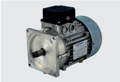
**Integral motors:** these are motors with a peculiar square flange and tang drive shaft, specifically engineered and manufactured for our mini power packs, featuring high power density and direct connection to the PPC central manifold. They are available in single phase or three phase execution, in frame 71, 80, 90 and 100, with square flange and tang drive shaft.
