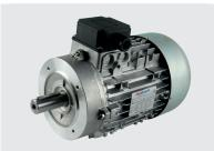
**B14 IEC motors:** for market compatibility, any IEC standard B14 AC motor with frame 63, 71, 80, 90, 100 or 112 can be mounted. These motors are normally procured and mounted by the customer himself. Two-piece couplings and additional adaptor flanges as per following tables must be fitted. Hydronit can supply frame 112 B14 AC 3-phase motors
