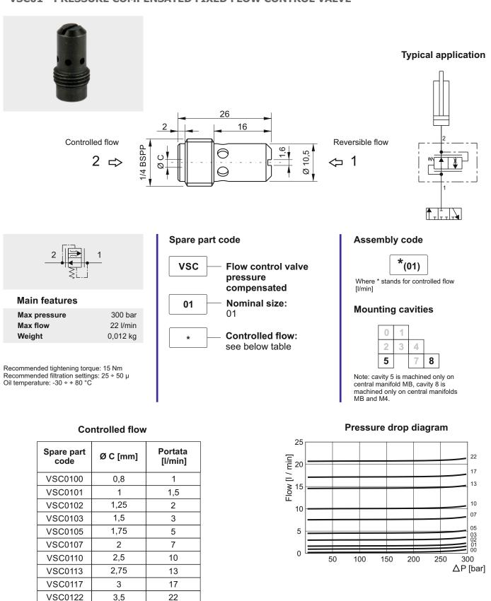
Note: nominal controlled flows, measured at 100 bar with an oil viscosity of 46 cSt at 50  $^{\circ}\text{C},$  are to be taken as general reference values and must be tested in the field.
