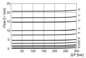
Note: Values measured on valve alone (no cavity) with an oil viscosity of 46 cSt at 50  $^\circ C.$  Pressure drop may change depending on fluid viscosity and temperature
