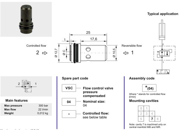
Mounting cavity dimension: 12,7 H8 Recommended filtration settings: 25  $\div$  50  $\mu$  Oil temperature: -30  $\div$  + 80  $^\circ\text{C}$
