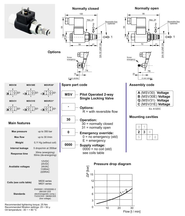
Note: Values measured on valve alone (no cavity) with an oil viscosity of 46 cSt at 50 °C. Pressure drop may change depending on fluid viscosity and temperature
